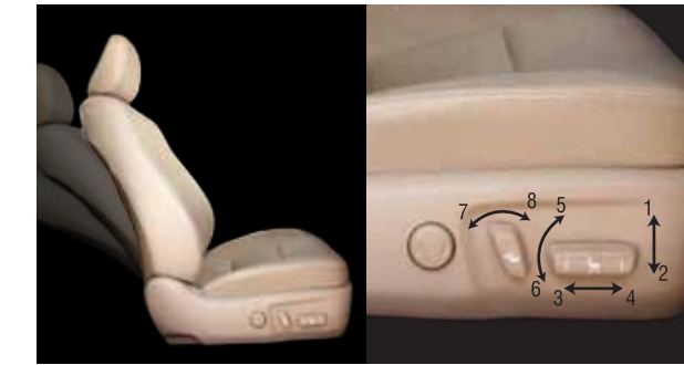
8-WAY POWER SEAT: Driver's seat with lumbar support, and co-passenger seat with Easy Access Function keys. Luxuriate in supreme, ergonomic, designer comfort.
